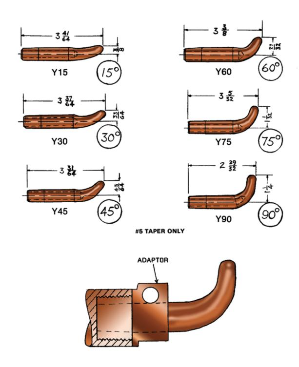
Radius Bend Electrodes are cold bent from 5/8 diameter RWMA Class 2 Bar Stock and are furnished with a 5/16 diameter water hole. They are used with an adapter that screws into a holder and clamps to the electrode. This arrangement affords a rigid assembly.
